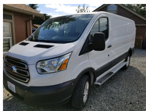
Cargo Vans 1 & 2 Inner box dimensions H:4'9" W:4'7" L:10'6"
