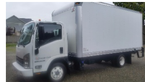
"White Bumper" Isuzu 16' Box Trucks with tilt up lift gate, rear exterior work lights, and back-up cameras.
