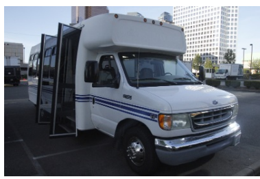
Shuttle bus -15 person with 2 exterior restrooms, VTR and DIGI-TECH Setup W/ 4K GENSET and Deep cycle Batteries
