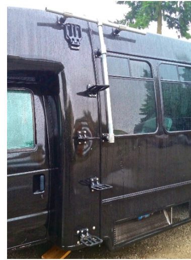
New ladder system on shuttle bus for attaching VTR antennas
