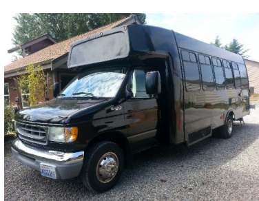
People Mover-15 person with 2 exterior restrooms, VTR and DIGI-TECH Setup W/4K GENSET, Deep cycle batteries and a 1000 Watt True Sine Wave Inverter.
