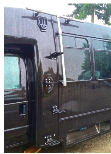
New ladder system on shuttle bus for attaching VTR antennas
